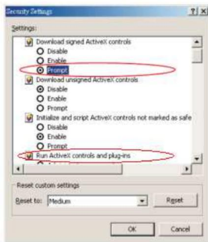
Once complete, you can access the IP camera's live video by entering the default IP address via your Internet browser. As the security warning dialog box appears, click **OK** to download the ActiveX directly from the IP camera.
