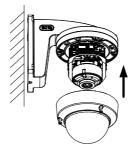
Figure 2-13 Install the Bubble
