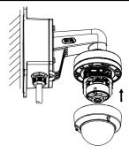
Figure 2-18 Install the Bubble
