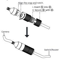
Figure 2-27 Water-proof Accessory Installation
