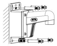
Figure 2-14 Fix the Bracket
