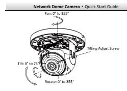
Figure 2-8 Angle Adjustment of Type III Camera
