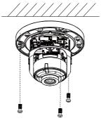
Figure 2-5 Fix the Mounting Base
