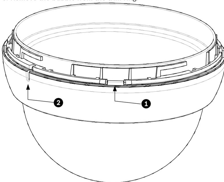
7. Insert the replacement bubble inside the trim ring and align the release tab (item 2, above) on the trim ring with the release slot on the bubble.
