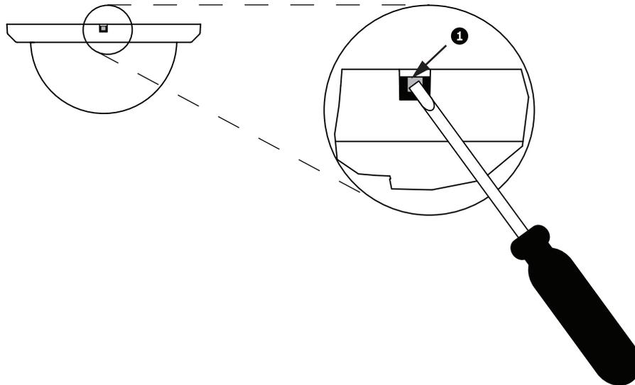
Figure 10.41: Bubble Release Screw
