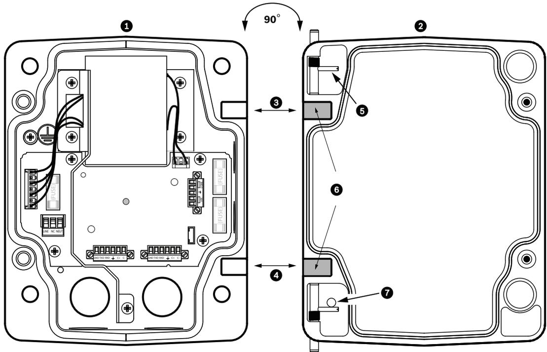
Figure 8.19: Align Cover Door Hinge to Power Box
