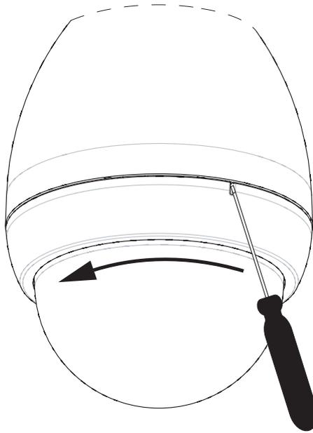
**Figure 10.42: Pendant Bubble Release Opening**
