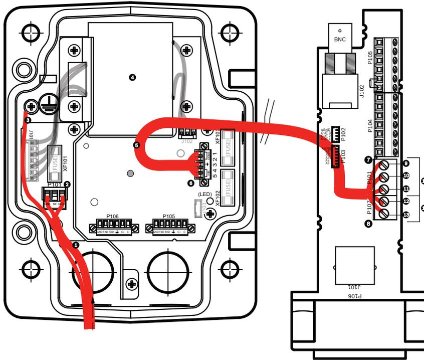
Figure 8.16: VG4-A-PSU1 or VG4-A-PSU2 Power Supply Box Connected to Pipe Interface Board
