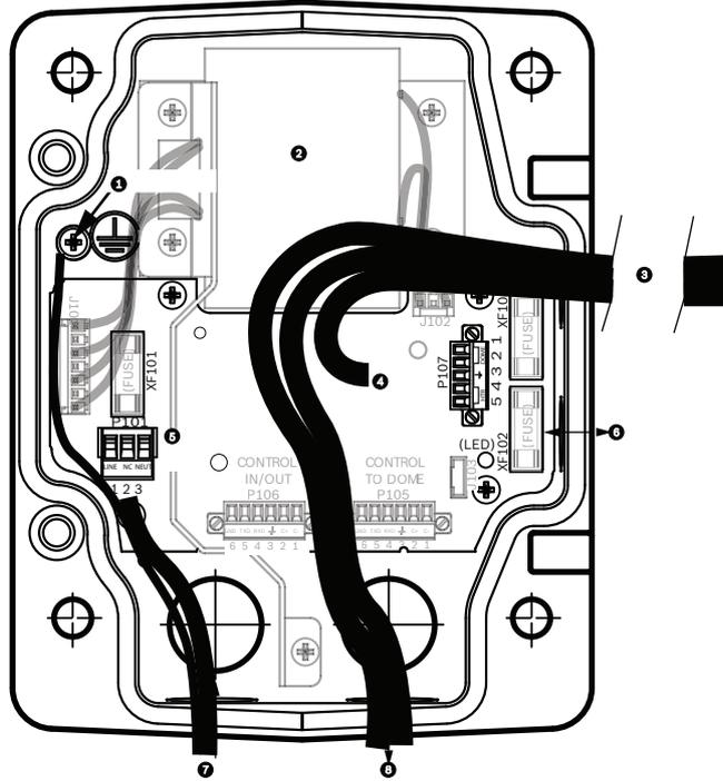
**Figure 8.18: Power Supply Box Connections**
