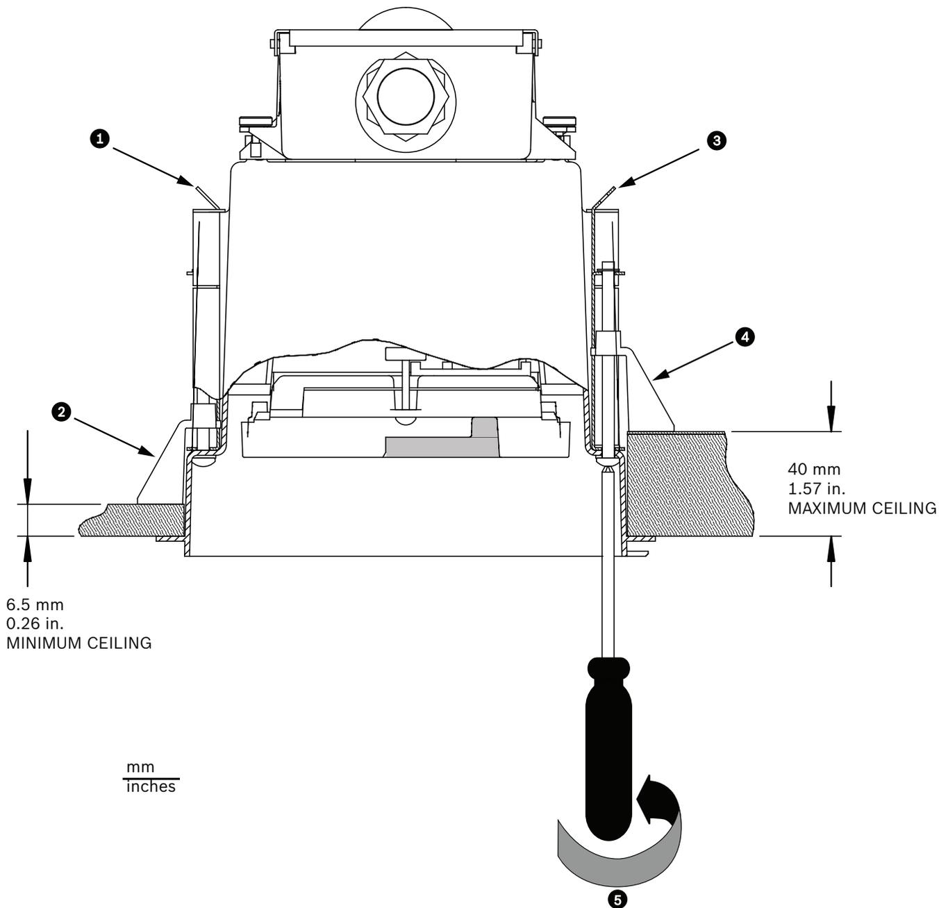
Figure 9.40: Secure camera to ceiling
