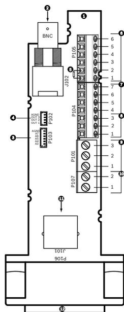
Figure 8.25: Pipe Interface Board Connections
