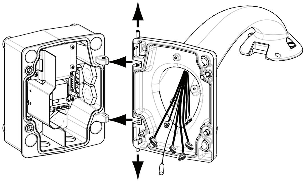
**Figure 7.9: Pendant Arm to Power Box Hinge Alignment**
