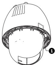
**Figure 5.1: Camera cross section with SD card slot**
