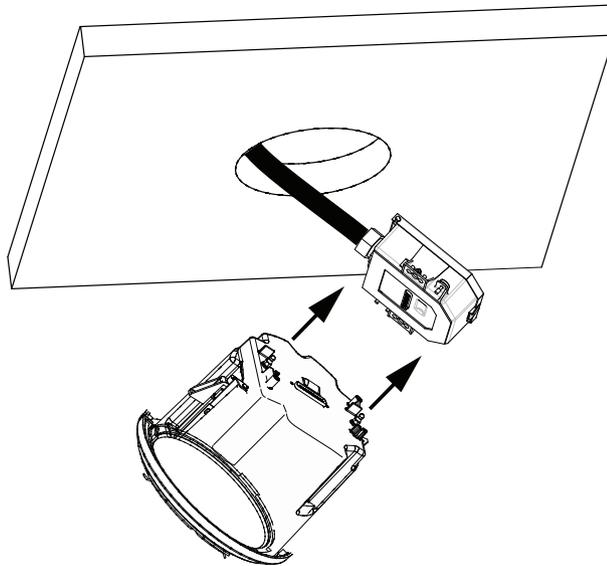
**Figure 9.38: Attach Housing to Interface Box**
