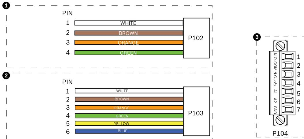
Figure 9.35: Alarm and relay connectors
