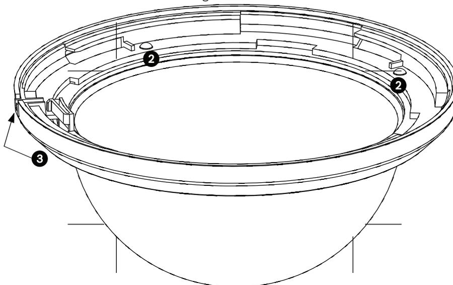
5. Remove the inner trim ring and remove the old bubble from the trim ring.
