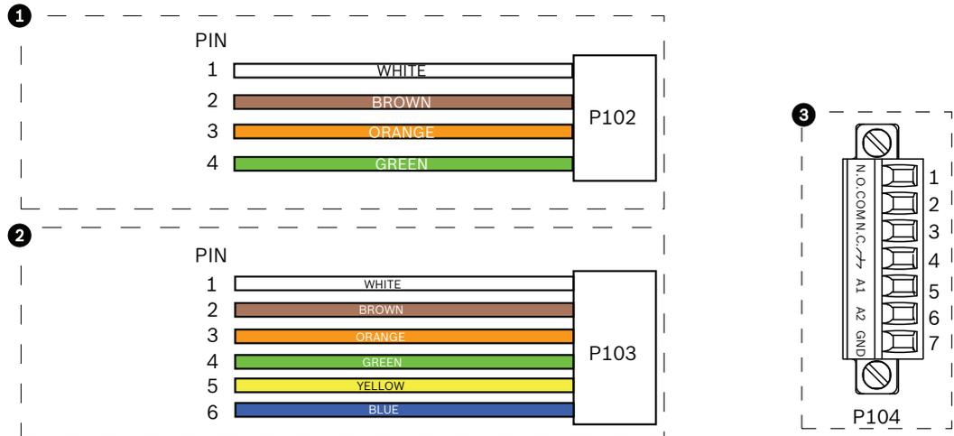
Figure 7.3: Alarm and relay connectors
