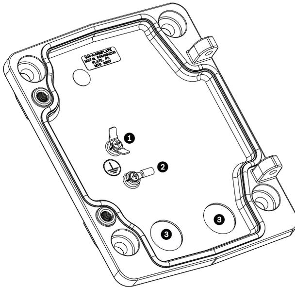
**Figure 7.13: Mounting Plate - Inside Detail**
