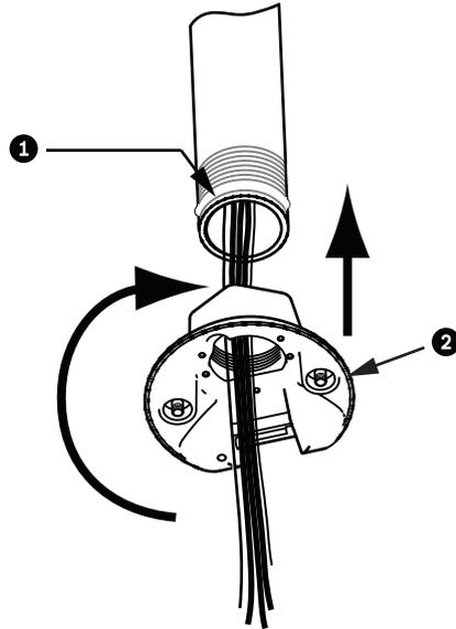
**Figure 8.23: Attach Dome Cap**
