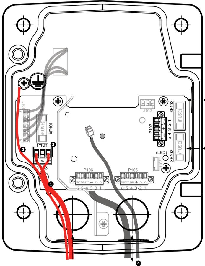
**Figure 7.8: VG4-PA0 Power Supply Box**
