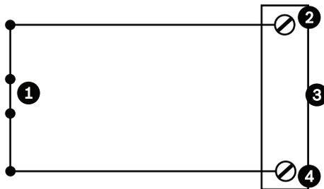
Figure 15.49: N.C. Normally Closed Non-supervised Connections
