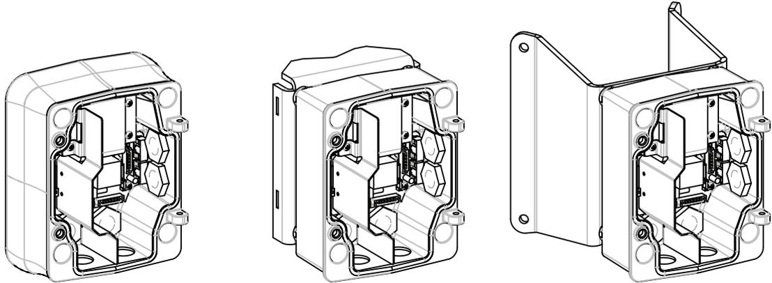
**Figure 6.2: Power Supply Wall, Mast (Pole), and Corner Mounts**
