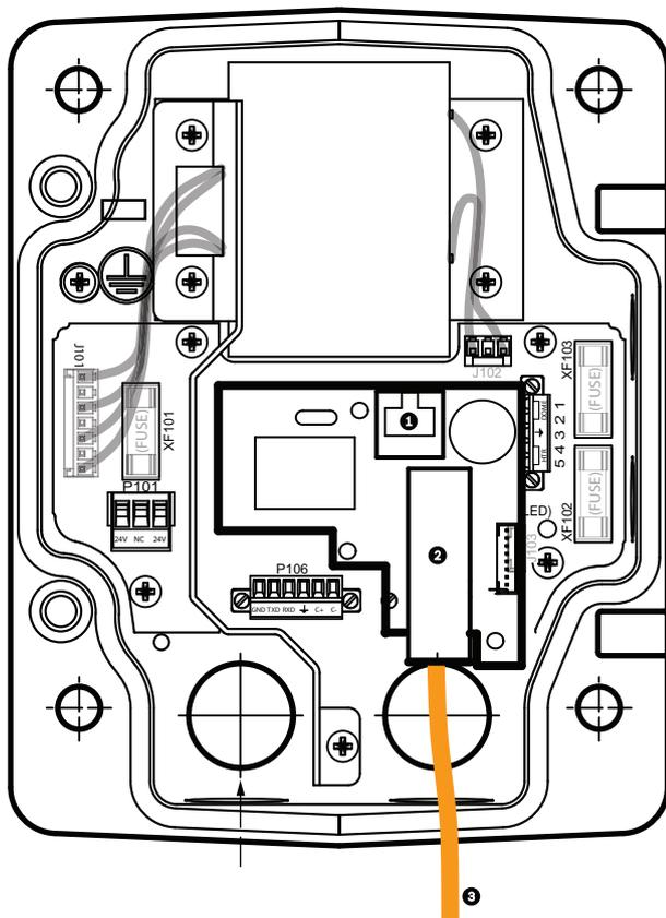
**Figure 8.17: Fiber Optic Ethernet Module installed**
