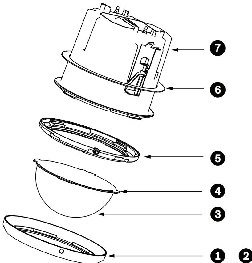
Figure 9.37: In-ceiling (IP54 Rating) Installation Diagram
