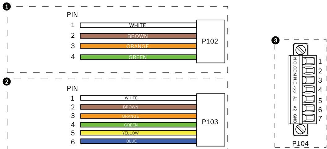
Figure 8.26: Alarm and relay connectors
