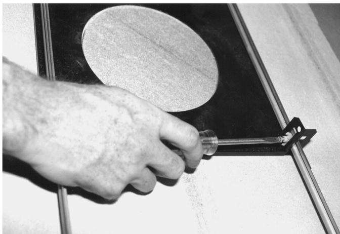
**Figure 9.32: Tighten Bracket Securing Screw**
