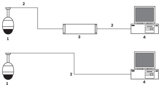
Figure 15.45: AUTODOME 7000 Series System Configuration
