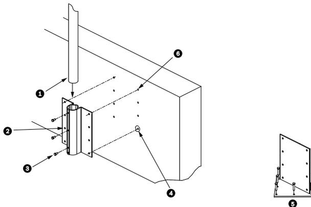
**Figure 8.21: Parapet Wall Mount Bracket and Roof Mount Plate**
