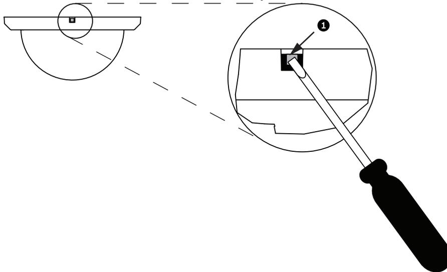
2. Rotate the bubble counterclockwise approximately 1/4 turn until it releases from the in-ceiling housing.
