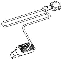
5. Attach the grounding spade from the 5-pin mating connector to the other spade terminal inside the mounting plate.
