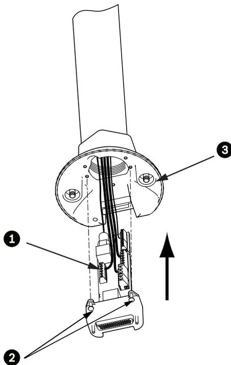
**Figure 8.27: Pipe Interface Board to Dome Cap Assembly**
