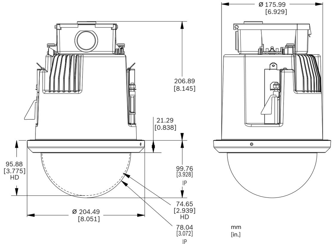
Figure 9.29: AUTODOME 7000 Dimensions – In-ceiling
