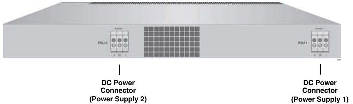
Figure 8. Back Panels of the Dual Power Supply Switches
