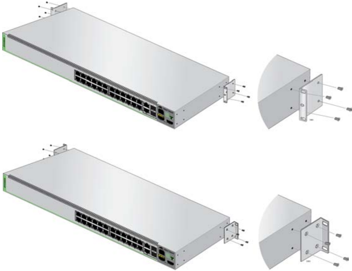
Figure 25. Attaching the Brackets to Install the Switch in an Equipment Rack (Continued)
