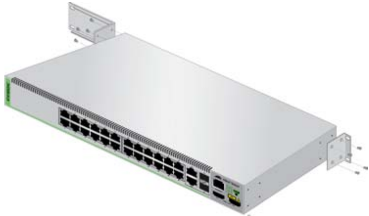
Figure 27. Attaching the Brackets to 8100L and AT-8100S/24C Switches for Equipment Rack Installation (Continued)
