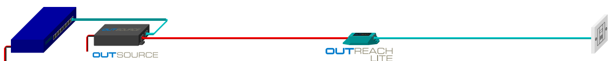
Example 2. If PoE is not already available, it can easily be added using Veracity's OUTSOURCE injector.
