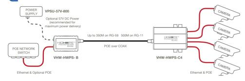
Connect 1-4 cameras or POE / non-POE devices to the RJ45 ports.
