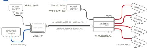
Connecting 57V DC power directly to the Quad unit increases the POE power available if required.
