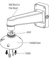
**2.** Turn the installation base in the direction of the arrow to join it to the mount.
