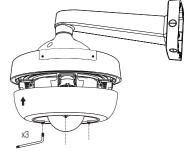
5. Join the installed base and the camera body by matching the Installation direction guides.
