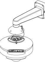
6. Turn the camera in the direction of the arrow so that the installation direction guides at the top and bottom are placed as shown below.
