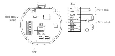
When the alarm output is connected as Normal Open:
