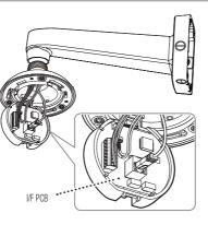
After fastening the I/F PCB to the body, install the safety wire of the camera body to the installed base.
