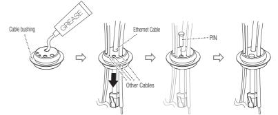
Inside the installation base, plug the cable bushing in the joint hole.
