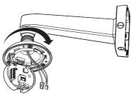
If the product is installed in an area where outside moisture can penetrate through the mount, use the provided cable bushing to block the inflow of outside moisture.
