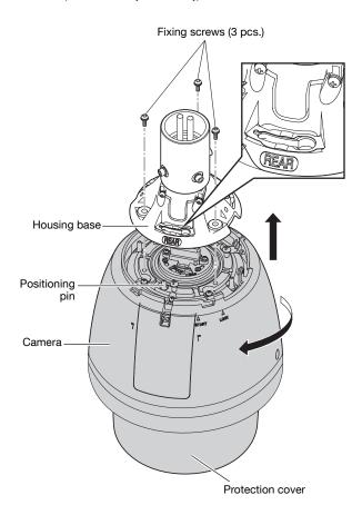
\* The illustration above is provided for describing the top of the camera, and therefore, this bracket is omitted.
