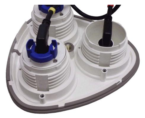
Fig. 15: Default front plate with sensor modules (back)
