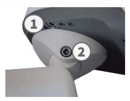
Fig. 72: Fastening the Camera
