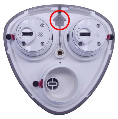
2. Push the front plate into the module housing until it stops.
