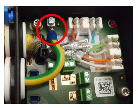
Fig. 66: Ground wire connected to terminal
