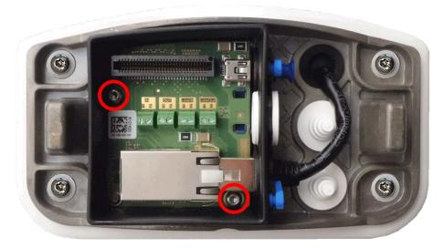
Fig. 55: Mount the Connector Box RJ45 (top view) using the two screws (highlighted red in the figure) on the mounting plate
