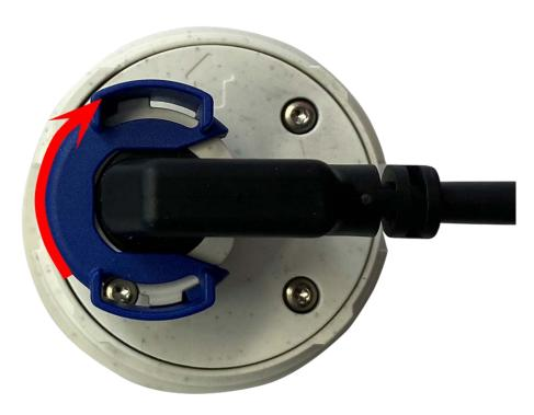
Fig. 11: Lock sensor module
