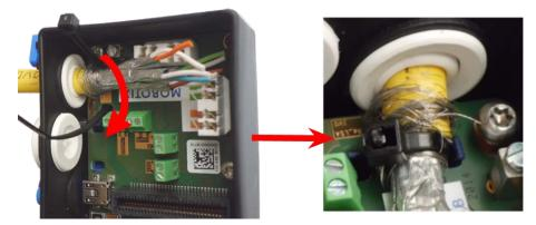
Fig. 61: Cable tie inserted beneath network cable
