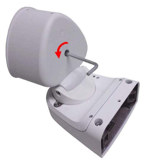
Fig. 14: Opening the module housing
