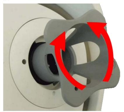
Fig. 84: Adjust lens focus
