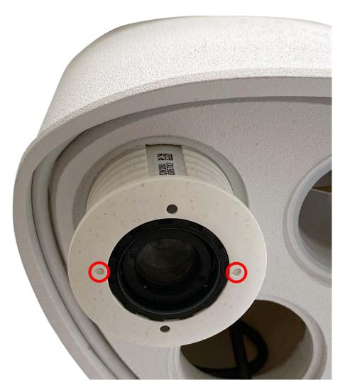
Fig. 12: Insert sensor module into module housing
