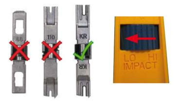
Fig. 62: LSA+/Krone tool set to LOW impact
