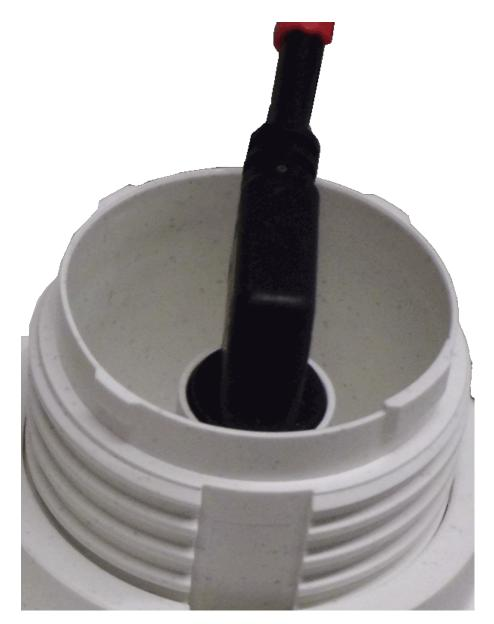
Fig. 10: Back of blind module with connector attached
