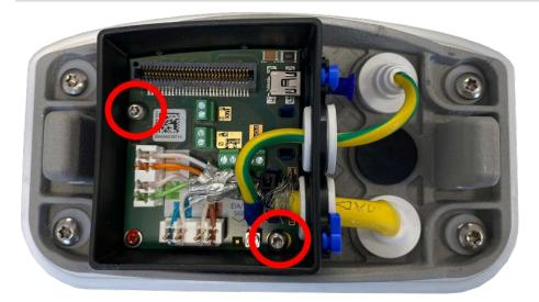
Fig. 67: Mount the Connector Box LSA (top view) using the two screws (highlighted red in the figure) on the mounting plate
