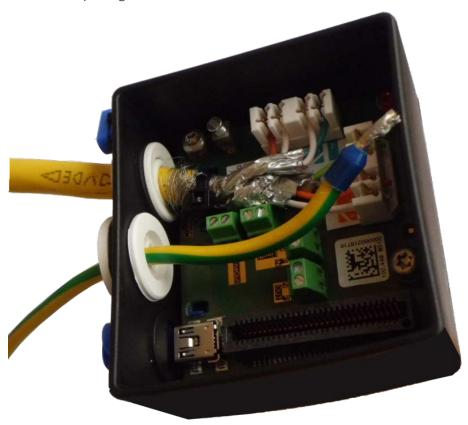
Fig. 65: Ground wire inserted, plug properly seated
