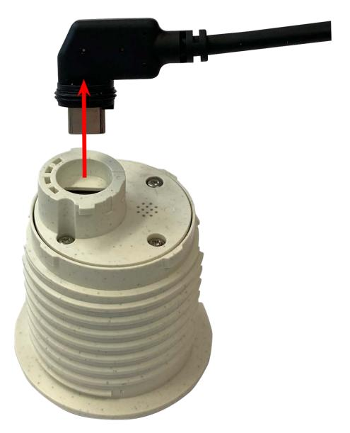
Fig. 21: Remove the sensor module cable
