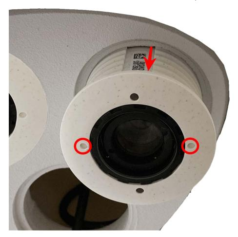
Fig. 23: Remove sensor module from the module housing
