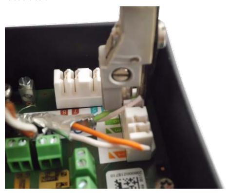
Fig. 63: Network wires connected using LSA+/Krone tool
