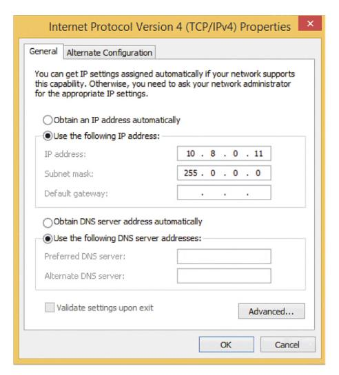
Fig. 76: Properties of Internet Protocol V4
