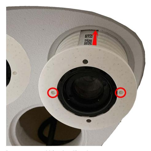
Fig. 25: Insert sensor module into Thermal front plate
