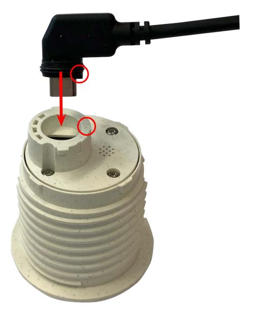
Fig. 9: Connect the sensor module cable
