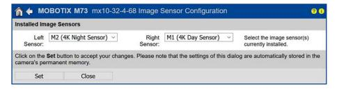
Fig. 89: Configuring the Sensor Modules
