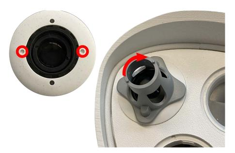
Fig. 13: Lock the sensor module
