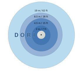
When mounted at a height of 3 m (10 ft) the  $180^{\circ}$  version of the camera has the following coverage radius for the four levels:
