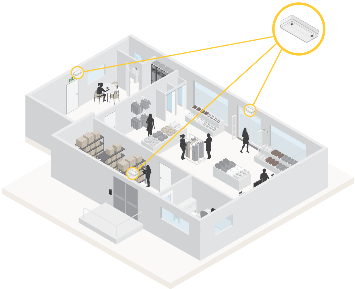
An example of a store with AXIS P8815-2 3D People Counter at each entrance.
