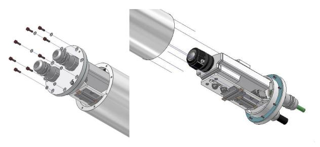
Fig. 6-3 Opening the ExCam XF Q1785 (similar illustration)
