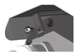
Fig. 6-1 Removing the weather protection roof (1/2) (this illustration is an example)
