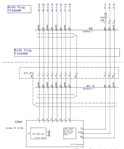
Fig. 5-4 Sample circuit of terminal box ExTB-3
