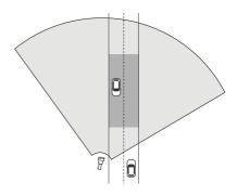
To measure high speeds accurately, position the radar within a lateral distance of 10 m (32 ft) from the vehicles. For more information about detection range and velocity accuracy, see *Road detection range on page 9*.
