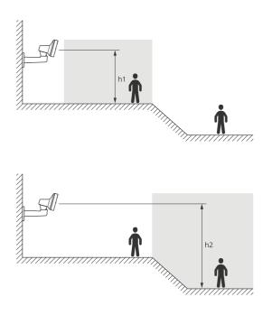
If the surface in the area of interest is uneven, add the average height (in this case (h1 + h2)/2) when you configure the radar.
