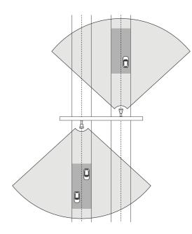
To measure high speeds accurately, position the radar within a lateral distance of 10 m (32 ft) from the vehicles. For more information about detection range and velocity accuracy, see *Road detection range on page 9*.
