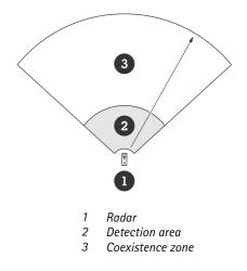
This radar operates on the 60 GHz frequency band. You can install up to eight radars operating on the 60 GHz frequency band close to each other, or facing each other, without causing problems. The built-in coexistence algorithm can find a suitable time slot and frequency channel that will minimize interference.
