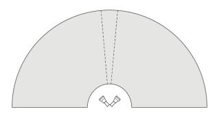
Two AXIS D2210-VE mounted side-by-side for 180° coverage.
