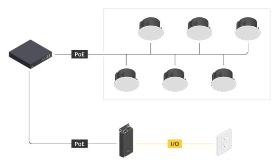
*Example: AXIS C8310 Volume Controller connected to a host device, which in turn is connected to the network. The system contains multiple speakers in a physical zone, but the host device does not belong to any physical zone.*
