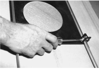
Figure 8.3: Tighten Bracket Securing Screw
