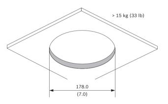
3. Pull the cables (24 VAC, CAT 5/CAT6, alarm and/or audio as needed) through the hole in the ceiling.
