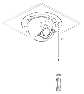
4. Tighten the clamps using the Phillips screwdriver to secure the housing to the ceiling.
