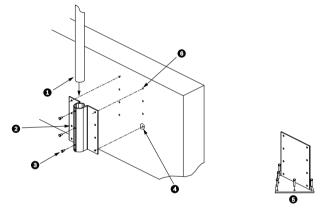
Figure 13.1: Parapet Wall Mount Bracket and Roof Mount Plate
