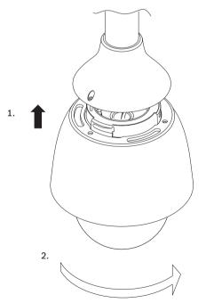
9. Secure the safety locking screw with the T15 Torx screwdriver.
